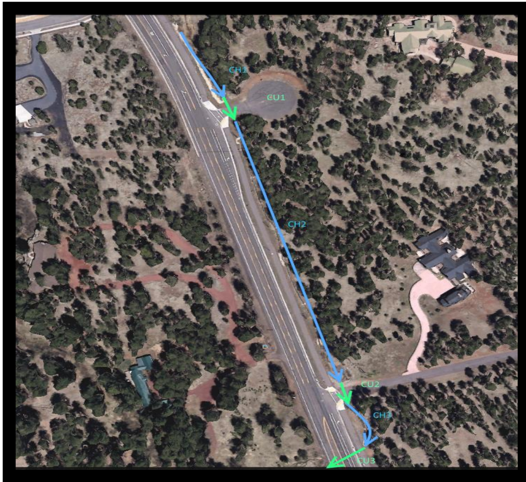
Figure 1: Aerial photo from Google Maps of Coyote Springs estate showing the channels and culverts on the reach
